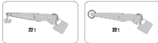
0,8 meters hook for reclinable boom head at -60° -30° 0°
